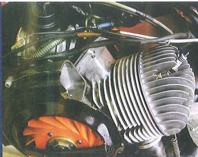
Piccio's experimental cylinder based on a Malossi barrel with a Cagiva reed block welded to it.
