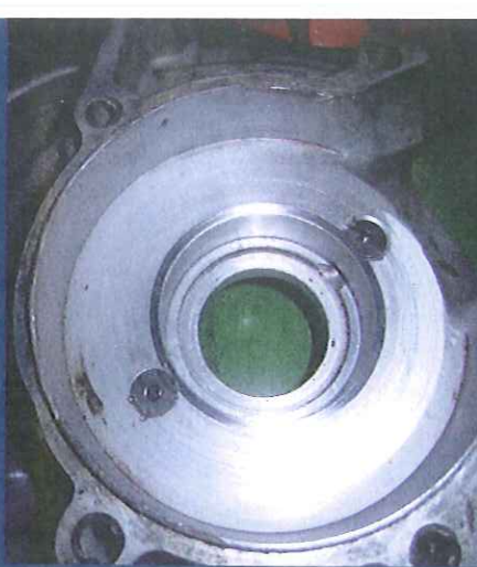
Lauro fits an adapter ring to the inside of the casings to allow the use of a better main bearing. The ring is retained by countersunk screws.
