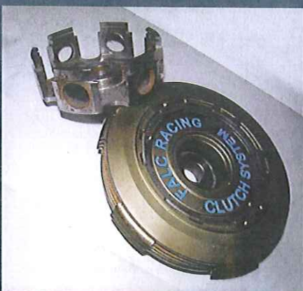
Falc parts are continually being upgraded. The next version of the small frame clutch will have a billet steel centre and improved clutch plates.
