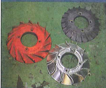
Lauro identified a problem with the fans for the popular Vespapronic and Parmakit ignitions. The orange Vespapronic fan blows well at low rpm but causes the air to cavitate (swirl around the fins rather than blowing) at high rpm resulting in insufficient cooling. The grey Parmakit one by contrast is too efficient and knocks over 3hp off the output of one of his race motors. His solution was to get a new fan CNC machined from aluminium billet that is designed to cool well without causing too much drag.
