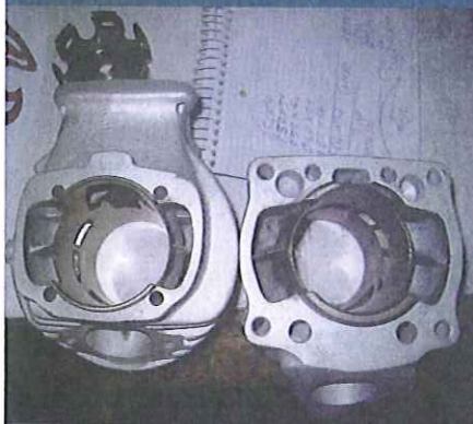
Comparing a Honda RS125 race cylinder to the 150 Falc kit. With the Vespa stud pattern it's not possible to add any more transfer port area.
