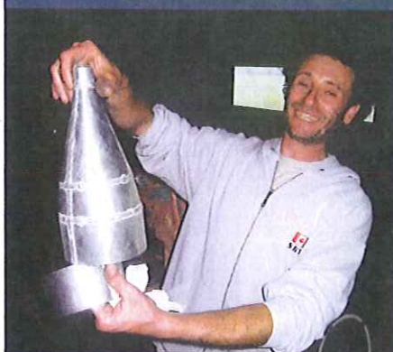
Lauro races 125cc hydroplanes. For those the exhausts are adjustable in length by foot control to widen the power band so he makes them from aluminium to save weight.
