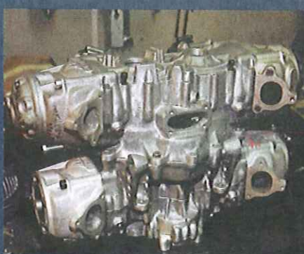
This is Lauro's new baby: a four cylinder 500cc two-stroke boat engine for world class hydroplane racing. He has designed and built it from scratch including the casings and the gears that connect the counter-rotating crankshafts.
