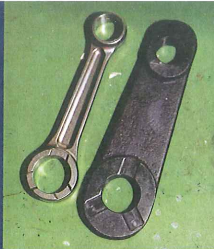
A blank forging and a finished con-rod which is tempered after machining. The Vespa rods are the same quality as the ones he uses for Grand Prix engines.
