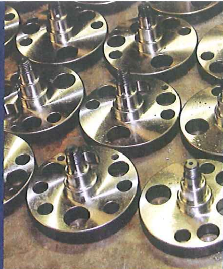
Forged crankshaft webs back from the machinist and ready for assembly and the fitment of balance weights.
